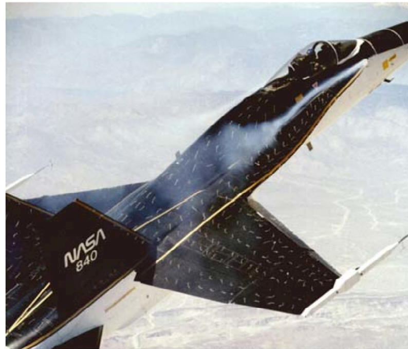
Dryden Flight Research Center EC89-0096-240 Photographed 1989 F-18 HARV smoke and tuft flow visualization. Angle of Attack = 30 deg. NASA photo.
