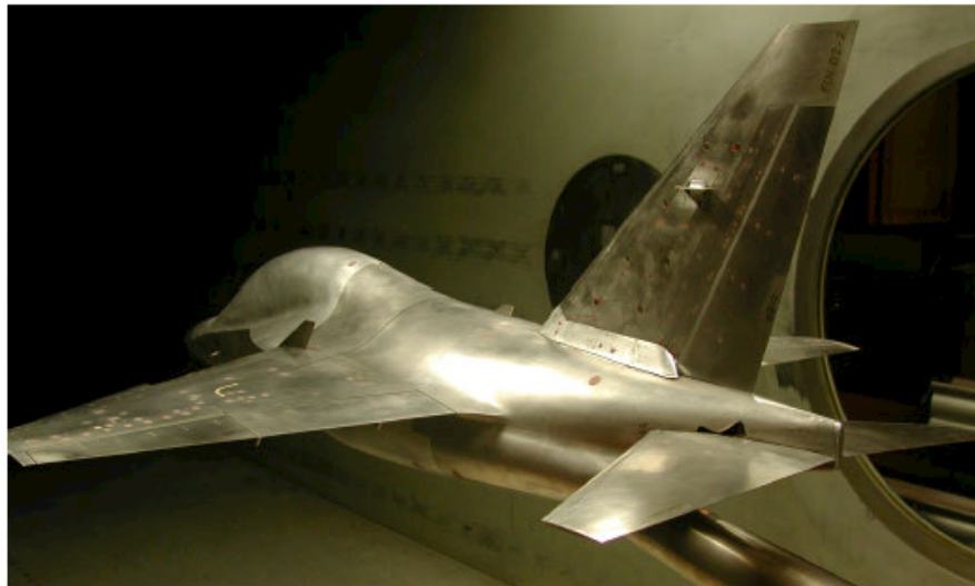
Fig. 4 Model D2, clean configuration, in DNW/HST wind tunnel
